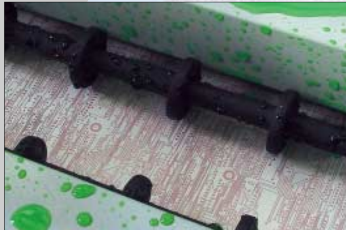
Blick in die Ätzkammer. A look into the etching chamber.
